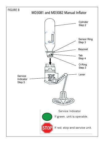
4) Raise, and hold, the lever into the inflator housing. Install a new cylinder/bayonet assembly by engaging bayonet tabs in housing, pushing in then turning clockwise 1/8 turn to a full stop (Fig. 9).
